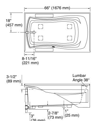
No change in measurements if connected with drain illustrated. (K-7161-AF) Recommended Faucet Location
